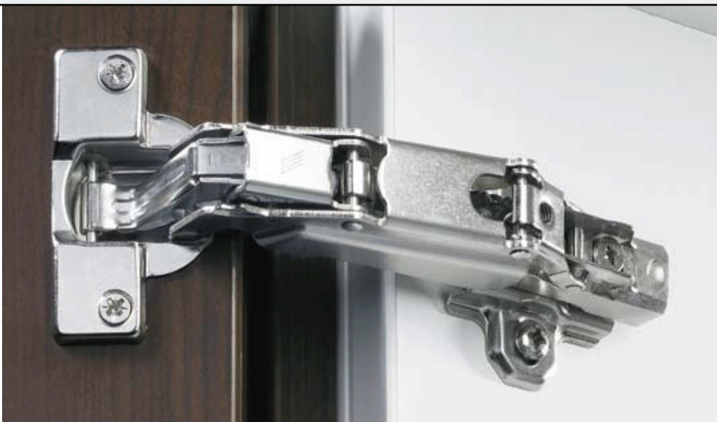
Interimat 9944 W-30 for negative 30° face angle Opening angle 125°
